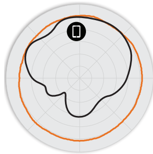
Figure 3. H510 5GHz Azimuth Antenna Patterns
